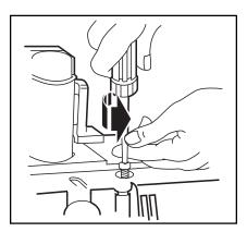
3. Turn Electroglide Powerhead over. To remove cover, insert screwdriver at cover tabs on both sides and twist to release tabs.
